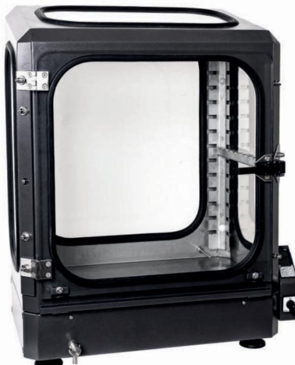
The resistance of coating materials to moisture is determined by exposing the test samples to condensation water.
