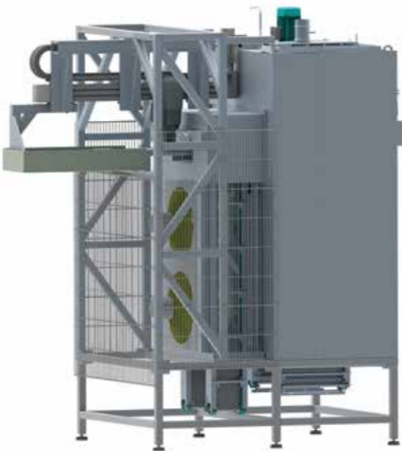
Integration in a customer on site transfer system | Heating zone with elevator stacking system | open cooling zone, cooling through axial fans Stacking furnace
